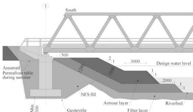
Fig. 9: Abutment detail
