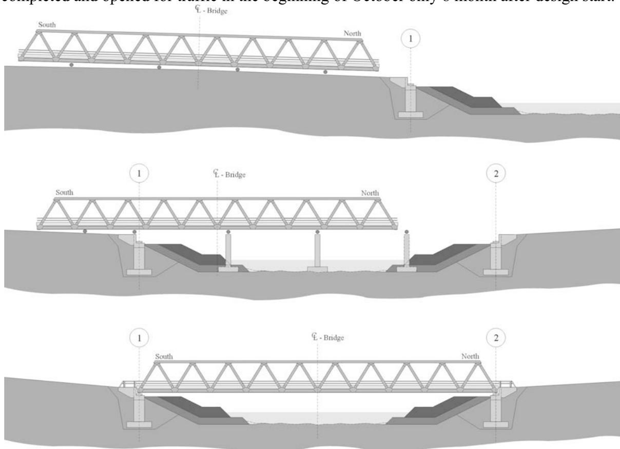
Fig. 10: Bridge sliding procedure
