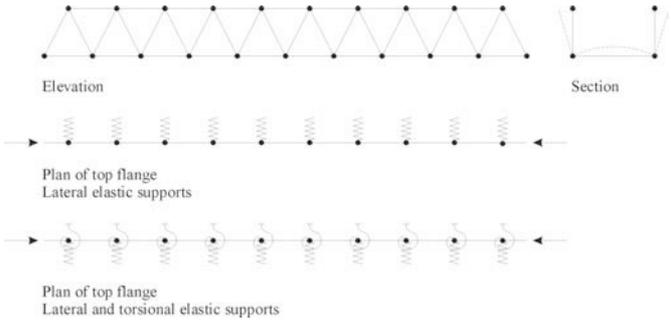
Fig. 7: Static model of top flange
