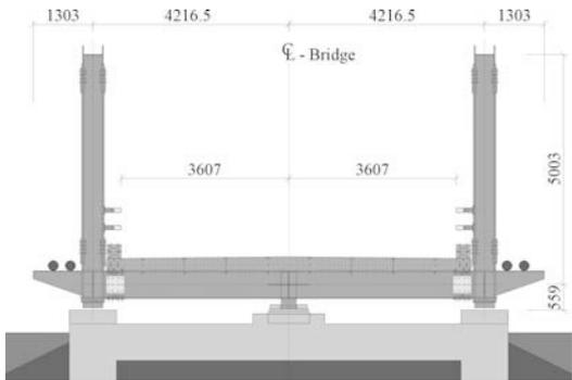
Fig. 4: Bridge cross section
