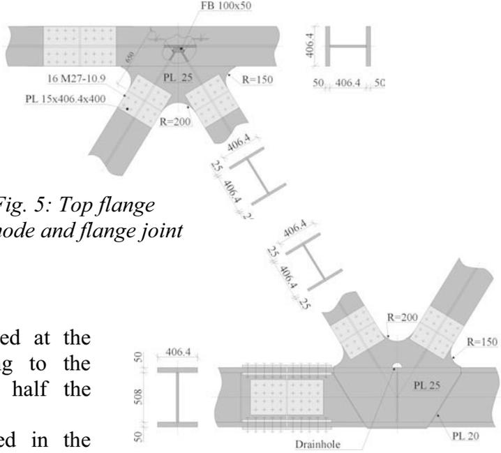
Fig. 5: Top flange node and flange joint
