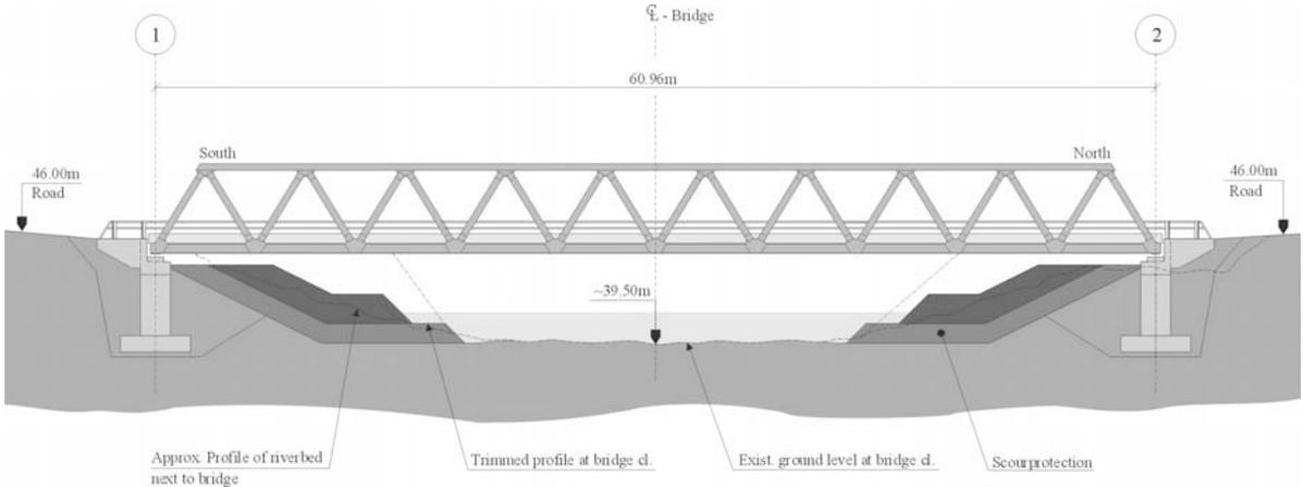
Fig. 2: Bridge elevation
