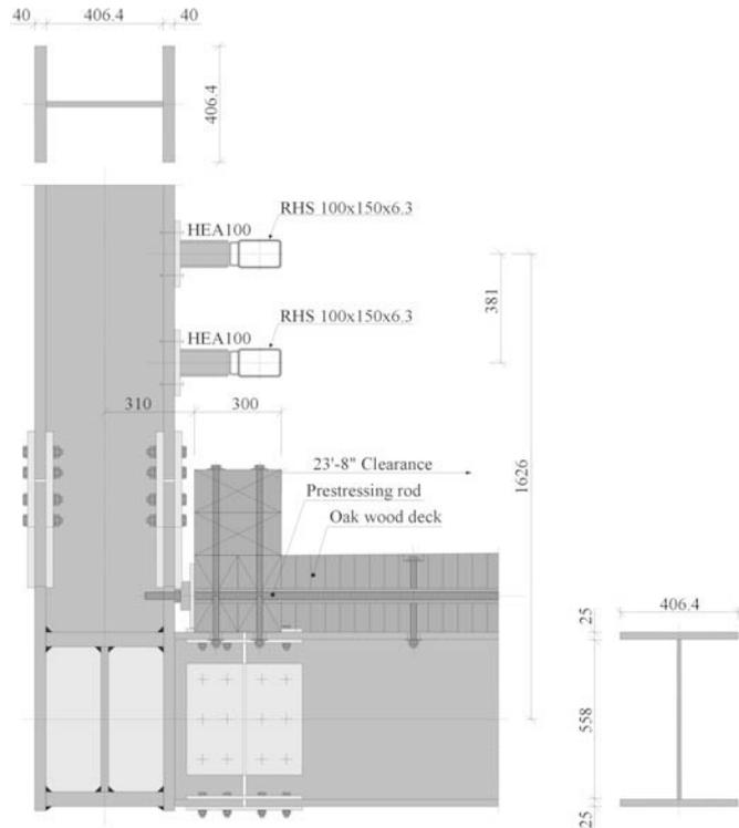
Fig. 8: Timber deck detail
