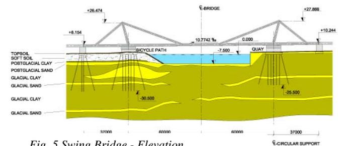
Fig. 5 Swing Bridge - Elevation
