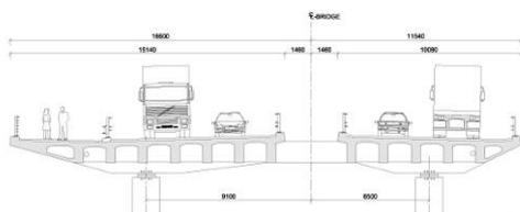
Fig. 4 Cross Section in Concrete Approach Span
